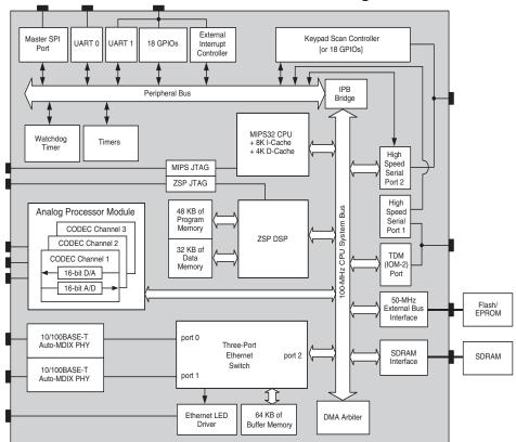
The Broadcom BCM1101 represents a new level of integration for feature enhanced Ethernet IP phone products.
